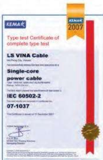
Type of cable : 19/33kV AL/XLPE/HDPE 1x300mm 2 Test Standard: IEC 60502-2:2005
